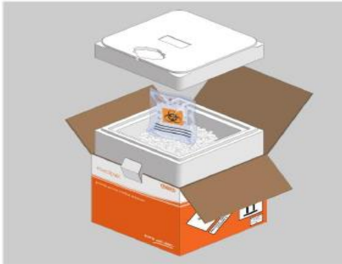
[3] Place the sealed pouch on top of the dry ice fill inside the insulating box. Apply the insulating box lid.
